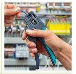
Stripping tool, for cable and conductors from 34 to 8 AWG, self adjusting, stripping length of up to 18mm with replaceable stripping blade.
